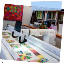
A programmable longarm machine used for finishing quilts.
